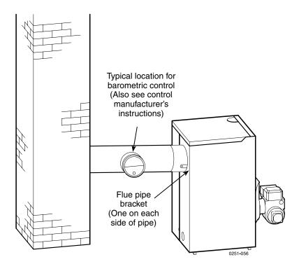
Figure 8 Top outlet breeching connection
