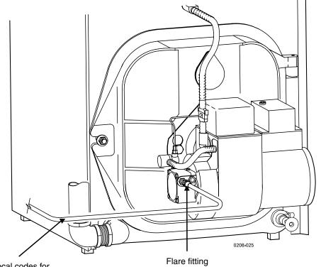
See local codes for appropriate arrangement and piping of filter control valves, etc., back to oil tank
