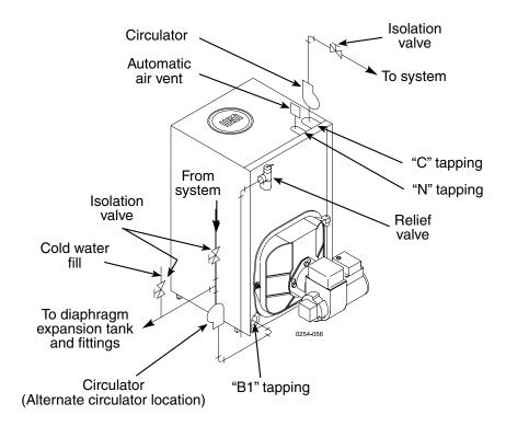
Figure 10 Piping with CLOSED expansion tank
